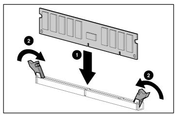
Figure 1-14: Installing a DIMM
